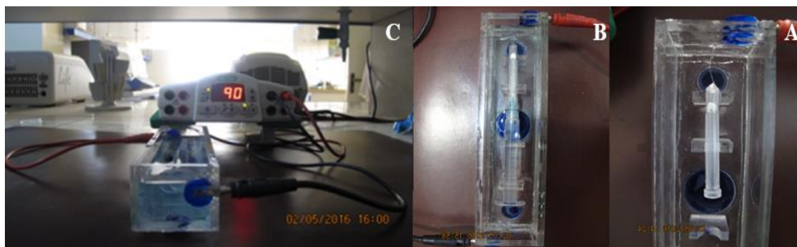
Fig. 2. (A): syringe needle cover. (B): Inserting the syringe cylinder containing the desired cut gene, connected to the 100 \mu l needle cover space through the syringe needle. (C): filling up the tank with TAE 1X buffer and connecting the invented device electrode to the electric power supply to perform gel electrophoresis at 90 V and 400 mA/gel for 7 minutes.
