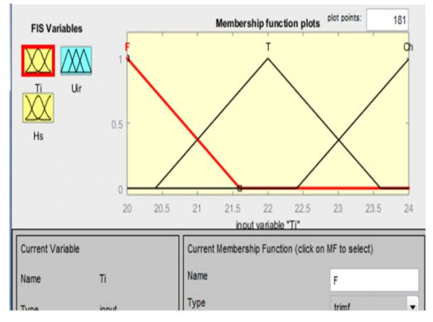
Fig. 1. (B) Current membership function for soil temperature inside the greenhouse.
