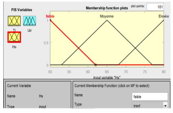
Fig. 1. (A) Current membership function for the soil humidity inside the greenhouse.
