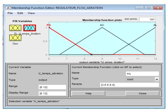
**Fig. 2.** (C) Membership function for the aeration as output.
