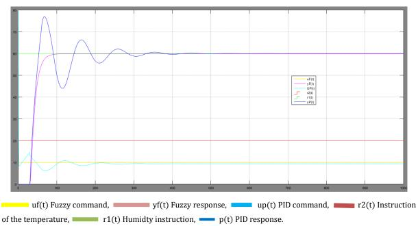
Fig. 4. Compared evolution of the numerical response functions for irrigation actions ordered by the PID controller
