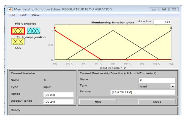
Fig. 2. (A) Membership function for the temperature Ti inside the greenhouse.
