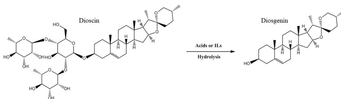
**Fig. 1. Dioscin hydrolysis process which catalyzed by inorganic acids or ionic liquids aqueous solution**
