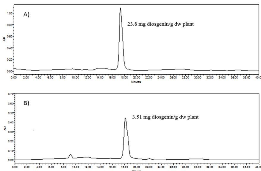
Fig. 4. Chromatograms of diosgenin (A) Boshruyeh ecotype with the highest content of diosgenin and B) Rafsanjan ecotype with the lowest concentration of diosgenin at 210nm. Column: HPLC C18. Mobile phase: Acetonitrile: water (90:10, v/v). Flow rate:  $0.4 \text{ ml min}^{-1}$
