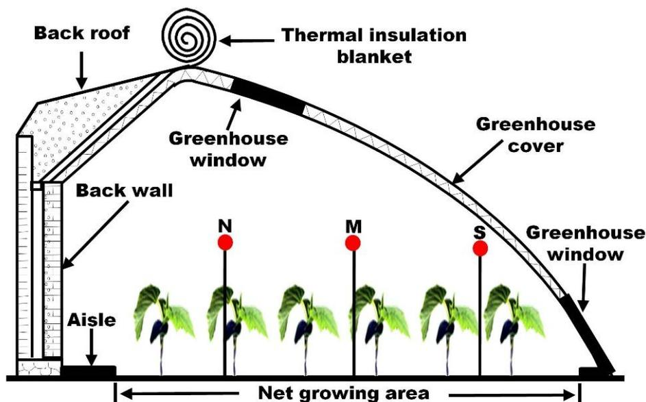
Fig. 1. Schematic diagram of cross section of Chinese Solar Greenhouse (CSG). N, M and S represent the location of quantum sensors for photosynthetic active radiation (PAR) measurements
