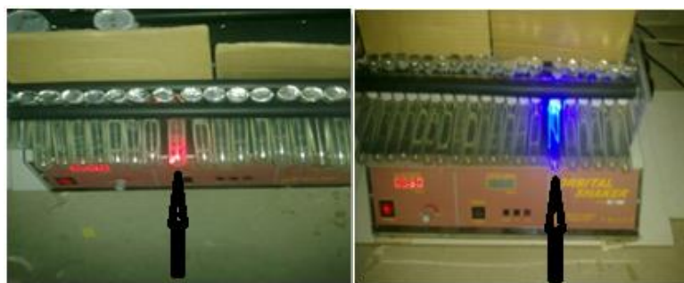
Fig. 1. Treatment of cell suspensions poured in L-shaped test tubes by red laser-He Ne (left) and blue laser-diode (right) lasers on a shaker
