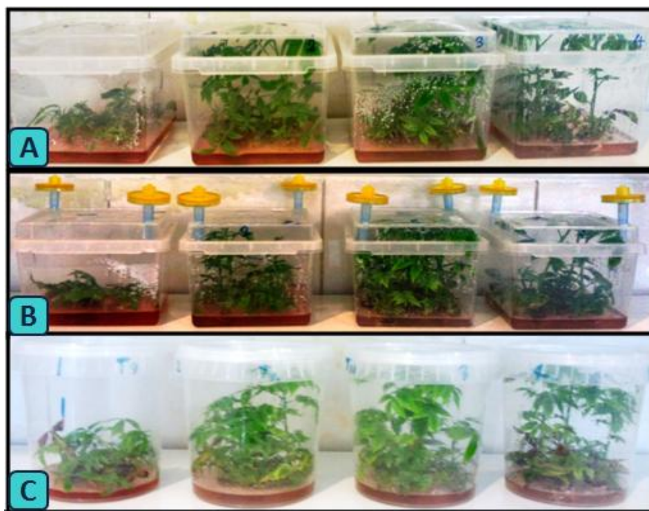
Fig.1. Walnut plantlets grown in non-ventilated vessels (A), type one ventilated vessels with two syringe filters on the lid (B) and type two ventilated vessels with 50 mm microporous polypropylene membrane (C) in a DKW medium containing 0, 15, 30 and 45 g L -1 of sucrose from left to right, respectively.
